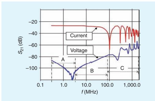
Fig. 14. Test performed on the calibration sample with one small circular aperture. The upper red curve shows the  $S_{21}$  vs the frequency when the input of the network analyzer is connected at the current probe. The blue curve below shows  $S_{21}$  when the N.A. input is collecting the near end voltage.
