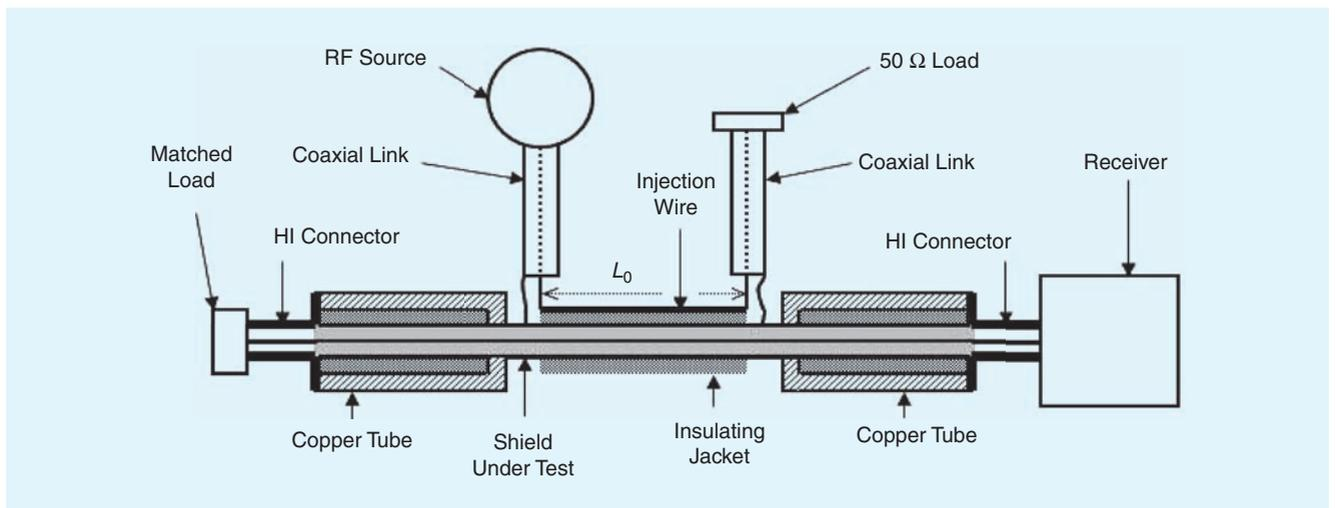
Fig. 1. Description of the wire injection setup.
