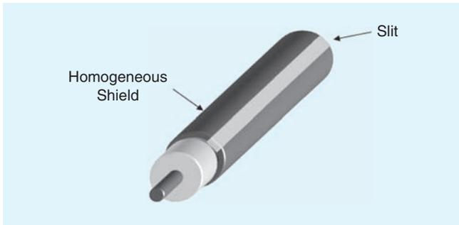
Fig. 3. Cable shield configuration with a slit.
